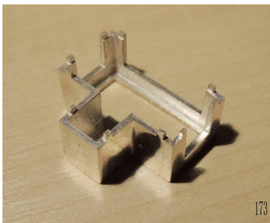
Fig. 172: The silver ring parts of 'Tu 凸' ring after 3D printing (Jiang, 2012).
