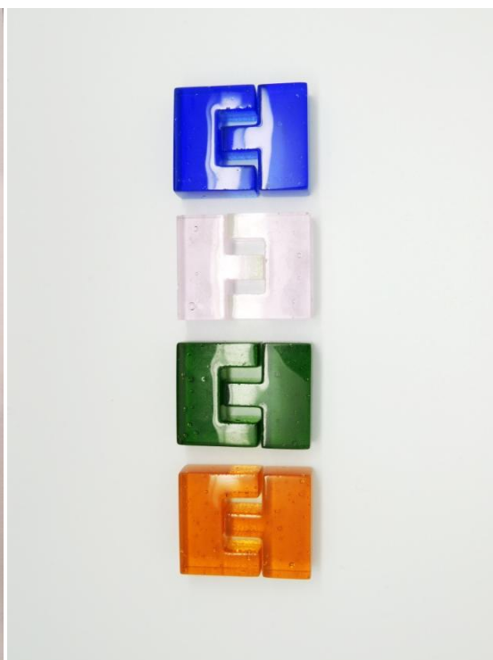
Fig. 179: Final four colours of 'Au Tu 凹凸' glass pieces after fire polishing (Jiang, 2013).
