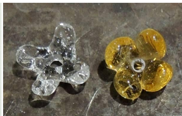
Fig. 131: The Osmanthus flower glass pieces made in yellow Soda Lime glass and clear Borosilicate glass by lampworking (Jiang, 2012).
