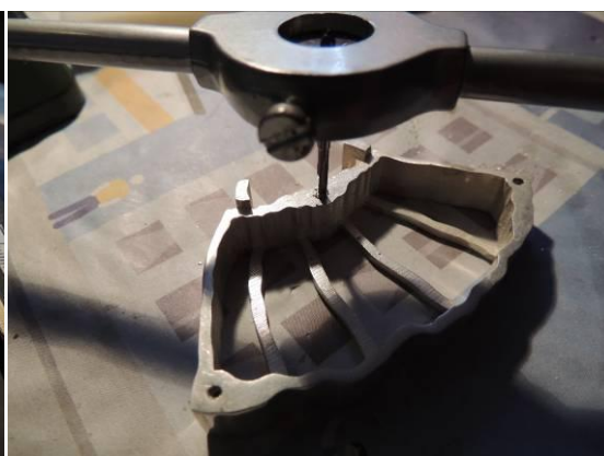
Fig. 306: Screw out the screw hole by tap and die (Jiang, 2012).
