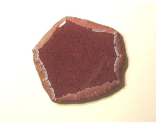
Fig. 230: The pentagon glass after fusing in the microwave kiln (Jiang, 2011).
