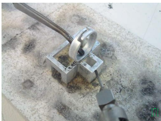
Fig. 171: Solder each silver parts of 'Tu 凸' ring (Jiang, 2012).
