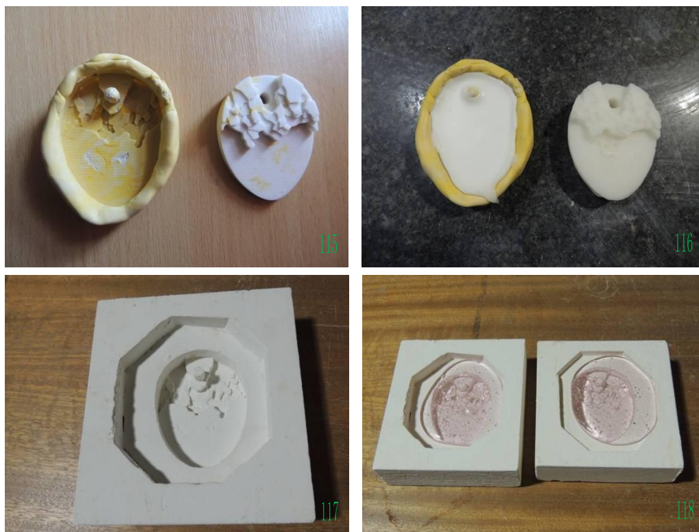
Fig. 115: 3D printing plastic 'Egg' to make 'Egg' mould putty (Jiang, 2012).
