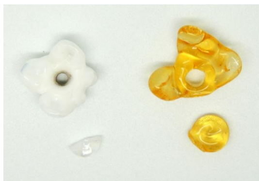
Fig. 130: The cracked Osmanthus flower glass by lampworking (Jiang, 2012).
