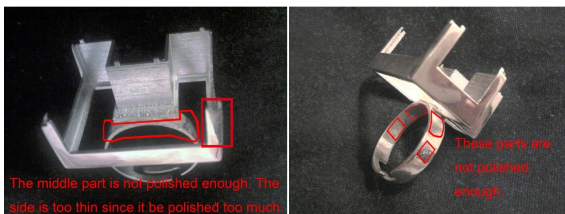
Fig. 60–61: The silver part making in my 'Ao Tu 凹凸' couple ring set (Jiang, 2012).
