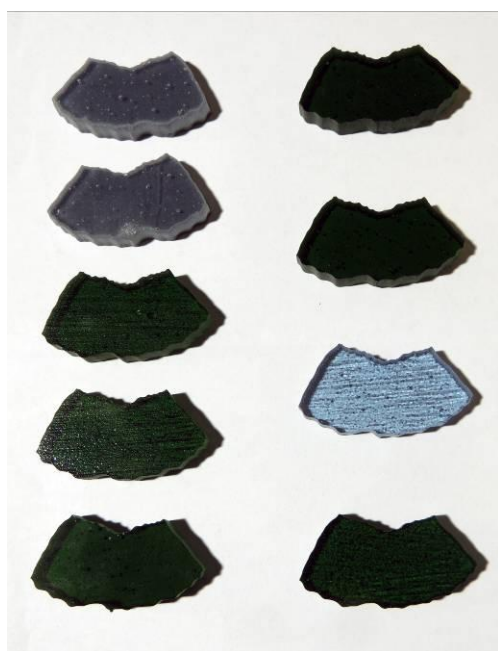
Fig. 309: Glass skirt pieces from water-jet cutting (Jiang, 2012).
