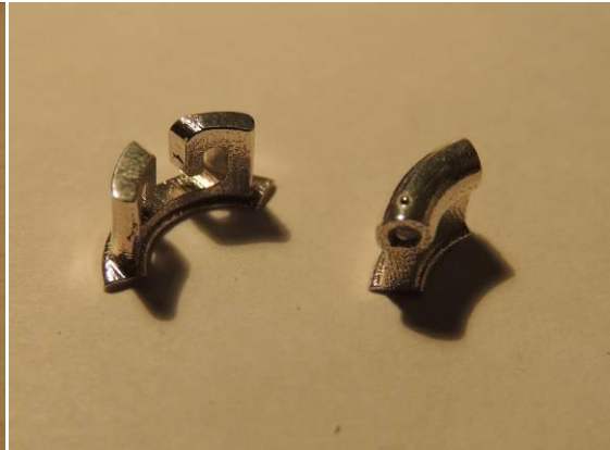
Fig. 252: The 3D printing of 'Button' brooch pin silver holder and protector (Jiang, 2012).
