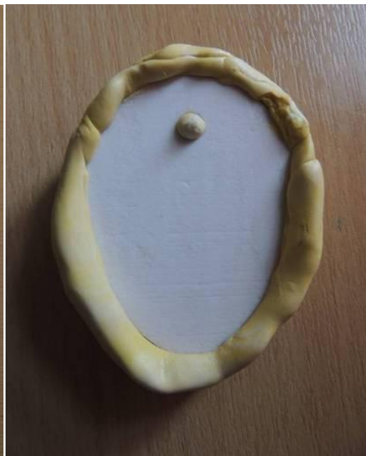
Fig. 206: Casting the white flexible plastic egg pendant into the mould putty (Jiang, 2012).
