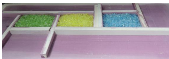
Fig. 107: Hammer Banas frits to prepare for fusing glass sheet in the kiln (Jiang, 2012).
