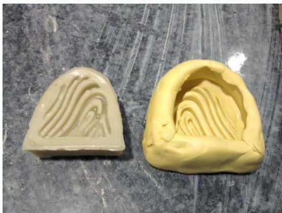
Fig. 331: The wax and mould putty of fingerprint (Jiang, 2012).
