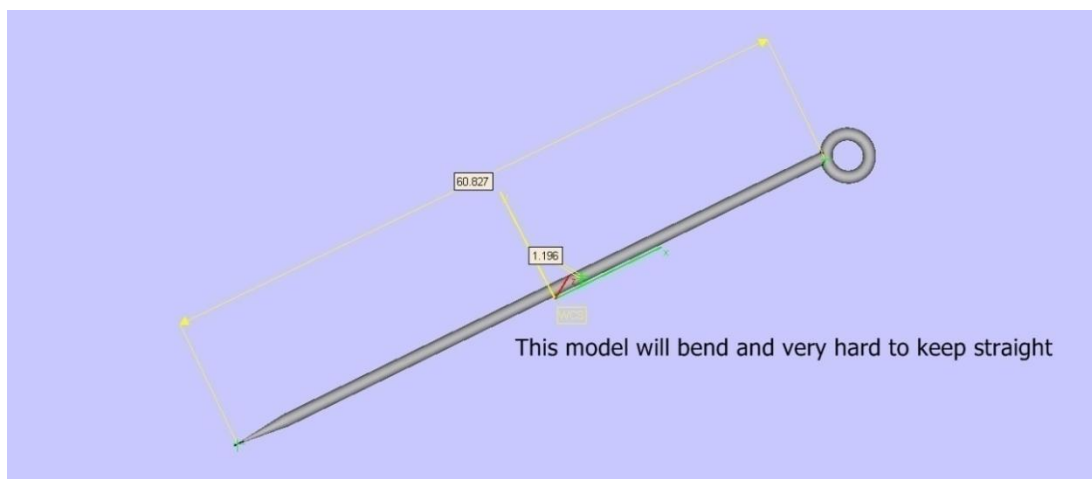
Fig. 87: The too thin and too long pin (Jiang, 2012).
