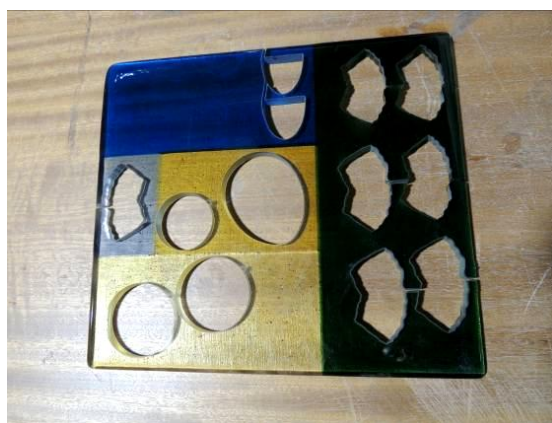
Fig. 102: Cut glass pieces separately (Jiang, 2012).
